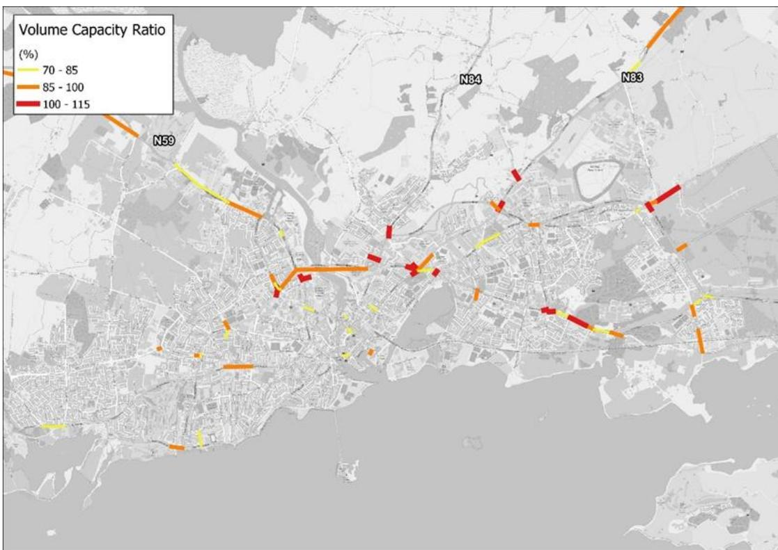
**Plate 3.15 Volume/Capacity Ratios at Junctions (2023 AM Peak)**
